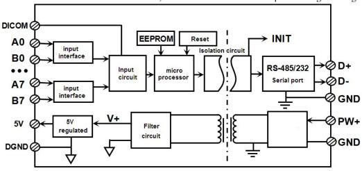
Figure 2: WJ69 Block Diagram
